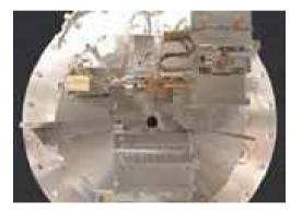
The positions of the two crystals in the instrument left are controlled to follow the orbit calculated by a computer. Multiple stages are used for position adjustment so that fine adjustment of Bragg angle and horizontal position adjustment of the beam are possible. Also the crystals are cooled with liquid nitrogen to withstand the thermal load of the beam. This instrument was installed at the Advanced Photon Source (APS) of the Argonne National Laboratory in the USA.
