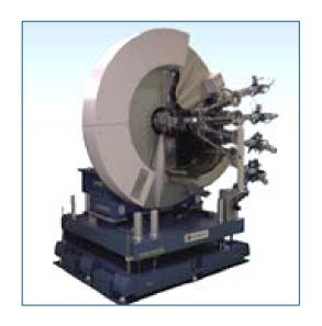
The diffractometer shown on the left is a specialized instrument for structural analysis of powder samples. An analyzer crystal and a detector are mounted on each detector arm. Only 15-degrees of rotation is required for measurement in an angle range of 60 degrees. This instrument incorporates MAX-G400 and MAX-G600. The axial coincidence of the  $\theta$ -2 $\theta$  axes is kept at approximately 5  $\mu$ m.
