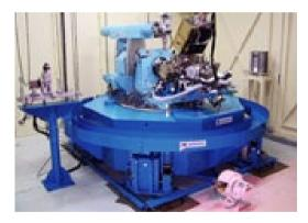
This diffractometer was manufactured for research of solid surfaces and thin film surfaces and interfaces. To observe the X-rays diffracted from the surface of a sample in any direction, this instrument has a four-axis structure comprising 2+2 axes.
