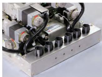
The 6-axis motor and sensor wiring are concentrated in one location to make even complicated multi-axis wiring work easy (can also be removed if not needed).
