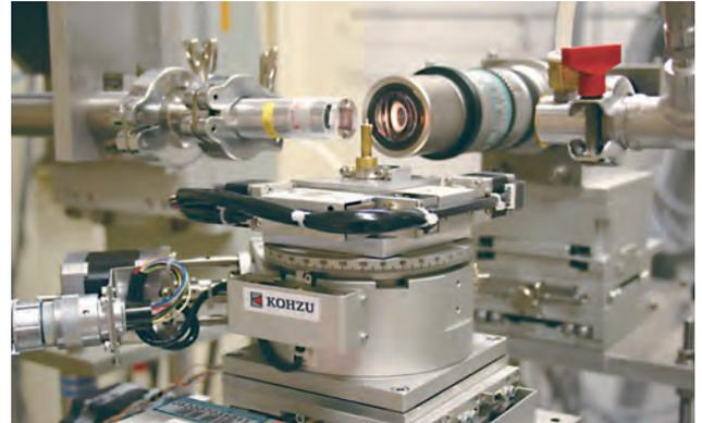
This Picture is shown as X-ray CT with SPU-1A for analysis of collected particle from Itokawa asteroid, Japanese Hayabusa mission (photo SPring-8).
